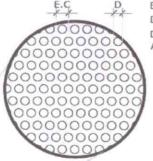
EC=13,8mm D=9,52mm DISPOSIÇÃO DOS FUROS: Alternada longitudinal
